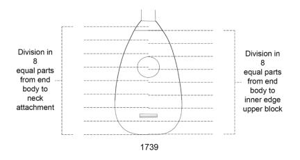
Drawing 5. The 1739 mandora soundboard comparing the equal division into 8 to the neck attachment (left) and to the inner-edge of the upper-block (right).
