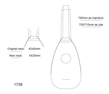
Drawing 6. The 1739 mandora with its current original neck (solid lines) overlaid with a 'new' lute neck (dotted line). Note how the upper-block changes to the same uniform results of the 1714 calichon and the 1726 mandora.
