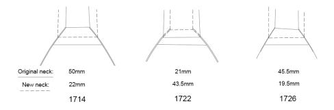
Drawing 4. Showing how large upper-blocks, normally fitted on lute moulds, were size-adapted for different instruments. Solid lines indicate the existing necks and upper-blocks, dotted lines indicate alternative necks applied to the same upper-blocks.
