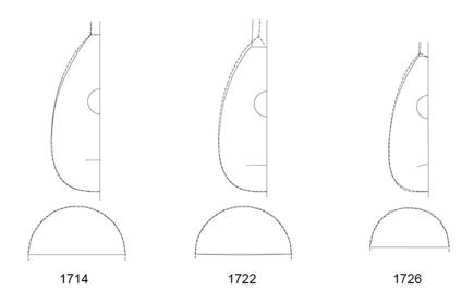
Drawing 1. Longitudinal and lateral cross-sectional views and soundboard profiles of Wenger's three earliest instruments.
