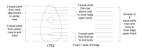
Drawing 11. The 1752 mandora, verification of the equal division in 8 to the inner-edge of the upper-block, which allows the rose center and bridge position to be checked as correct. Other internal structures were not accessible.
